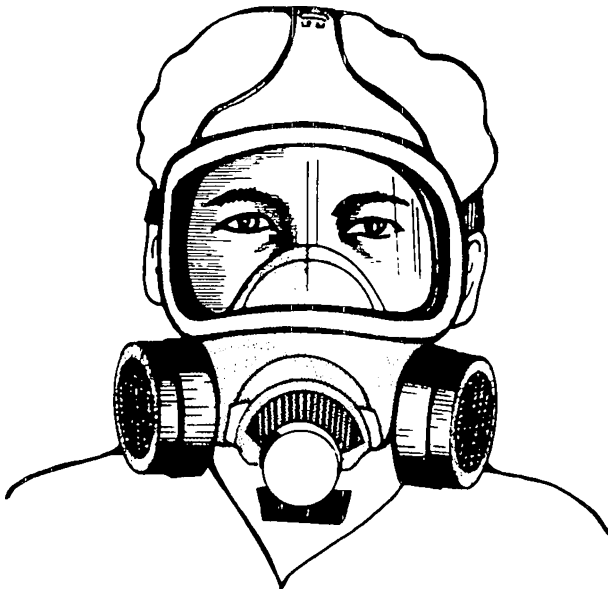
FIGURE 9 FULL-FACE PARTICULATE FILTER (CARTRIDGE) RESPIRATOR
