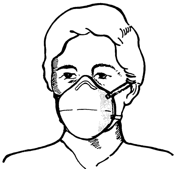
FIGURE 6 DISPOSABLE, HALF-FACE PARTICULATE RESPIRATORS
