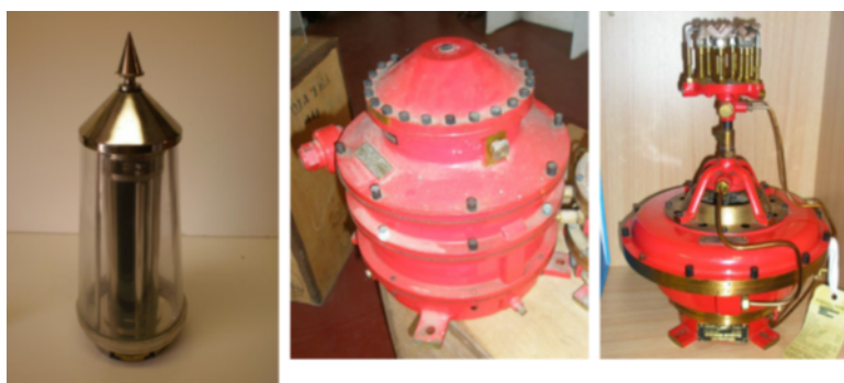
Figure 10. Dalén's system - sunvalve, mixer and flasher (Source: AMSA)
