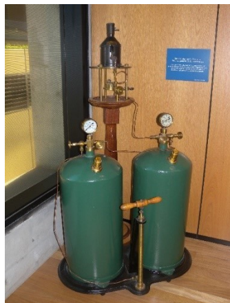
Figure 7. Incandescent oil vapour lamp by Chance Brothers (Source: AMSA)
