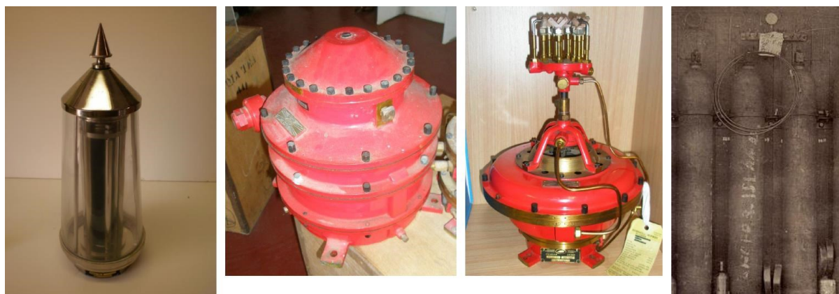
Figure 9. Dalén's system – sunvalve, mixer, flasher and cylinder (Source: AMSA)
