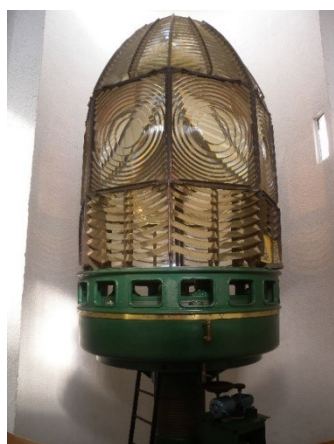
Figure 8. Dioptric lens on display at Narooma (Source: AMSA)
