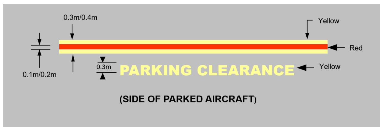
Figure 8.50 (5) Parking clearance line (shows matters)
