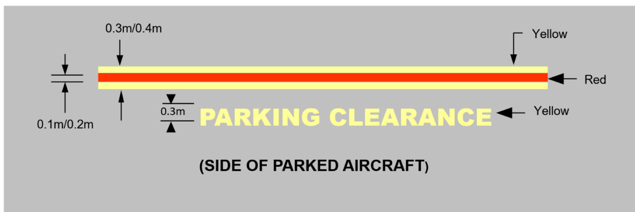
Figure 8.50 (5) Parking clearance line (shows matters)
