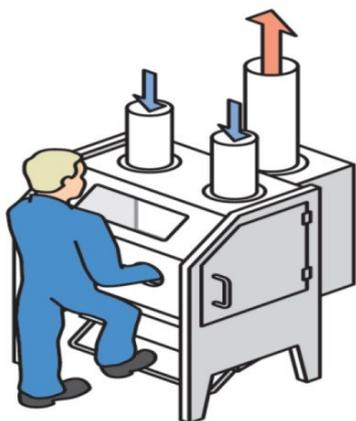
**Diagram 2** Side hood ventilation for an open surface tank
