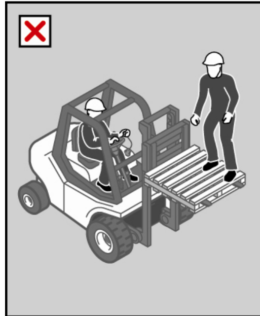
Figure 13: Using a forklift as a working platform or to gain extra height by standing on the tynes or a pallet is an unacceptable practice.
