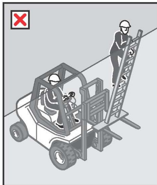
Figure 14: Unacceptable practice with ladder on forklift.
