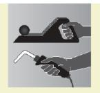
Select tools that can be held with a neutral wrist or in a handshake position with the hand adopting a comfortable (not too open or too closed) grip. Orient jigs and fixtures holding the workpiece so that the wrist does not have to bend.
