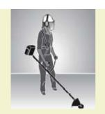
The heaviest part of this brush cutter is located behind the wrists and the weight is supported by a harness.
