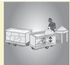
A self-adjusting base in the laundry tubs reduces the need for bending, twisting and reaching during unloading.
