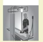
An overhead suspension system reduces the forces required to use the iron.
