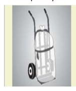
A trolley can eliminate many of the risks involved in manual handling, however, the load will still need to be manoeuvered onto the trolley and through the workplace.
