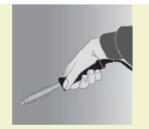
Excessive bending of the wrist is required to use this tool.
