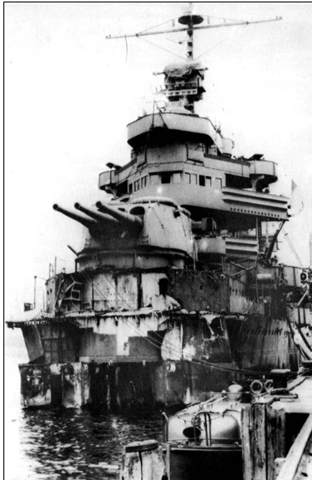
Figure 19: Fifteen United States Navy ships were repaired at Cockatoo Island during WW II. Included among them was the USS New Orleans, which was torpedoed in the Battle of Lunga Point, losing 150 foot of its bow in the ensuing explosion. The New Orleans steamed backwards from the Solomon Islands to Cockatoo where a temporary bow was fitted. This allowed the ship to return to the US for reconstruction.
