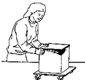
Figure 44 - Rolling platform to avoid lifting
