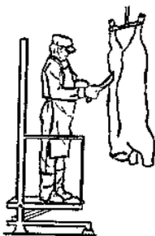
Figure 25 - Adjustable platform reduces stooping and reaching
