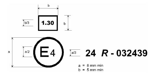
The above approval mark affixed to an engine/vehicle shows that, pursuant to Regulation No. 24, the engine/vehicle concerned has, with regard to the emission of visible pollutants by the engine, been approved in the Netherlands (E 4) under approval number 032439; the Regulation, at the time of approval, included already the 03 series of amendments. The corrected absorption coefficient is 1.30 m<sup>-1</sup> (in the case of a vehicle approval).
