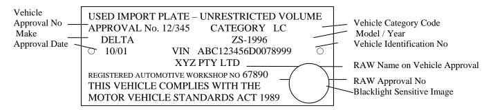
Dimensions 95mm x 35mm (approx) 2 x 3mm holes on horizontal Centre Line (for metal plates)
