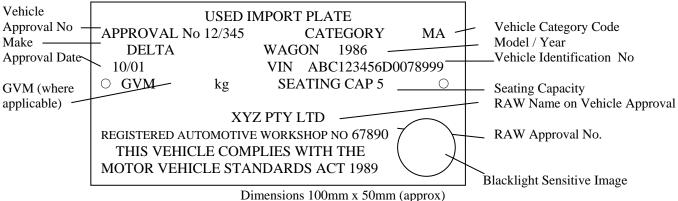
2 X 3mm holes on horizontal Centre Line (for metal plates)
