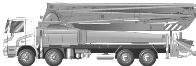
Figure 2 Illustrative example of a mobile concrete pump
