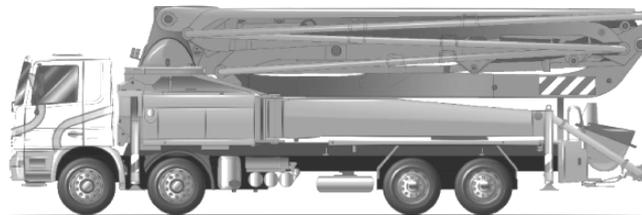
Figure 2 Illustrative example of a mobile concrete pump
